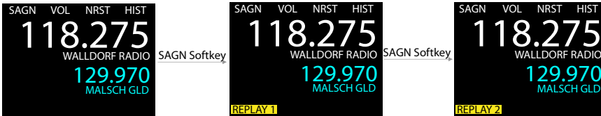
Figure 4.19.: SAGN softkey has been pushed, replay function is active and SAGN softkey is pushed again to replay an earlier transmission.
