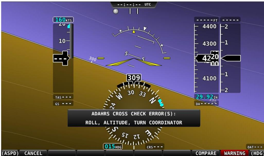
Figure 36 - ADAHRS Cross-Checking Disagreement
