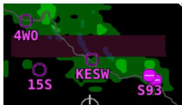
Figure 117 - Missing NEXAD Data Blocks
