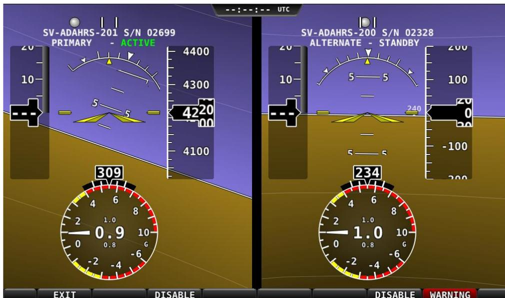
Figure 37 - ADAHRS Cross-Check Comparison
