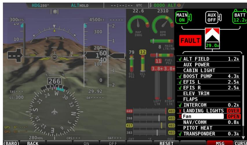
Figure 58 - VP-X Page with Fault
