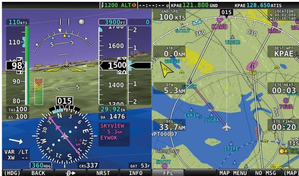
Figure 105 - Active Flight Plan: Map and Flight Plan View
