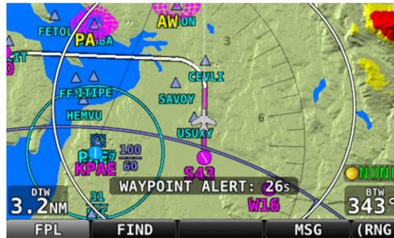
Figure 104 - Flight Plan Alert Messages
