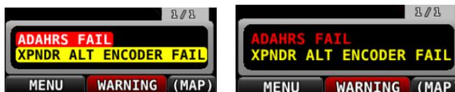
**Figure 176–Unacknowledged (left) and Acknowledged (right) Alarms**
