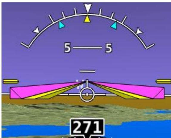
**Figure 164 - Single Cue / Inverted-V with Autopilot Servos Engaged**
