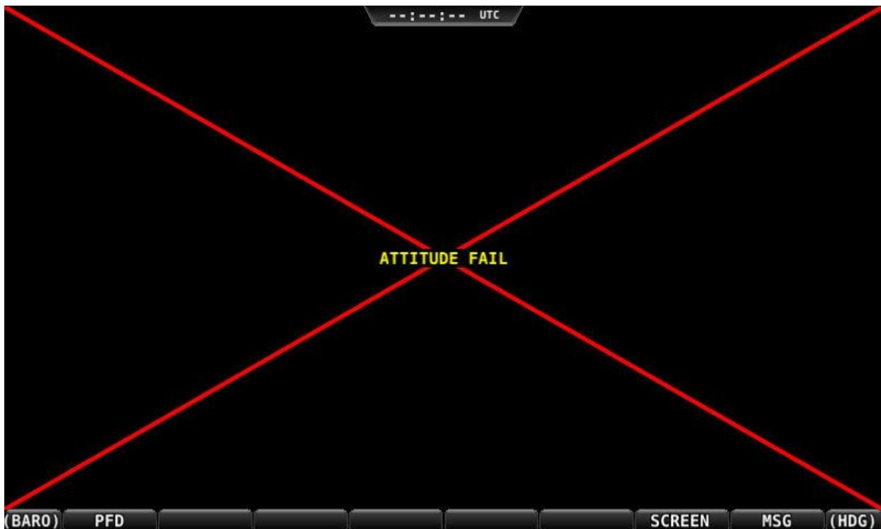
Figure 173–Example SkyView Failure
