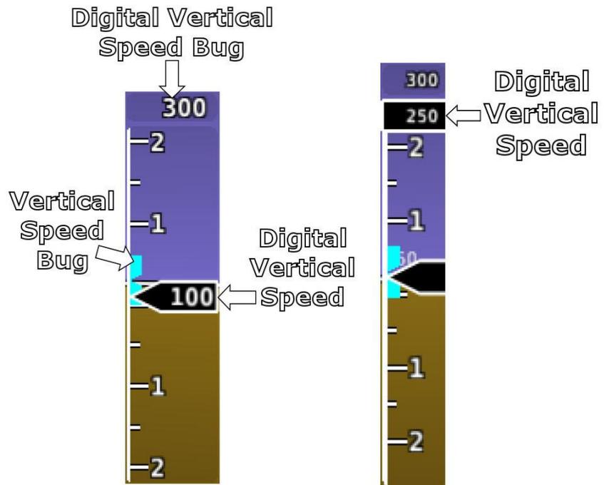
Figure 20—Example Vertical Speed Indicator.
