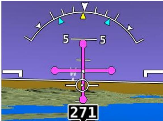
Figure 166 - Dual Cue / Cross Bars with Autopilot Servos Engaged
