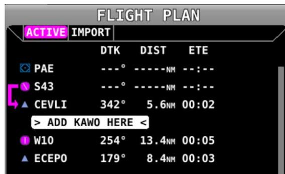
Figure 103 - Flight Plan Waypoint Insertion
