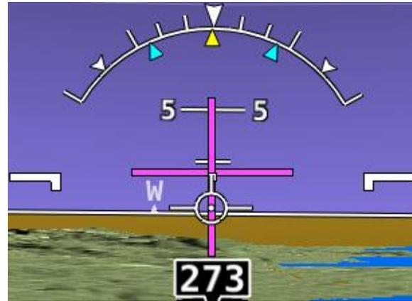
Figure 167 - Dual Cue / Cross Bars with Autopilot Servos Not Engaged
