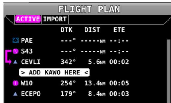
Figure 103 - Flight Plan Waypoint Insertion
