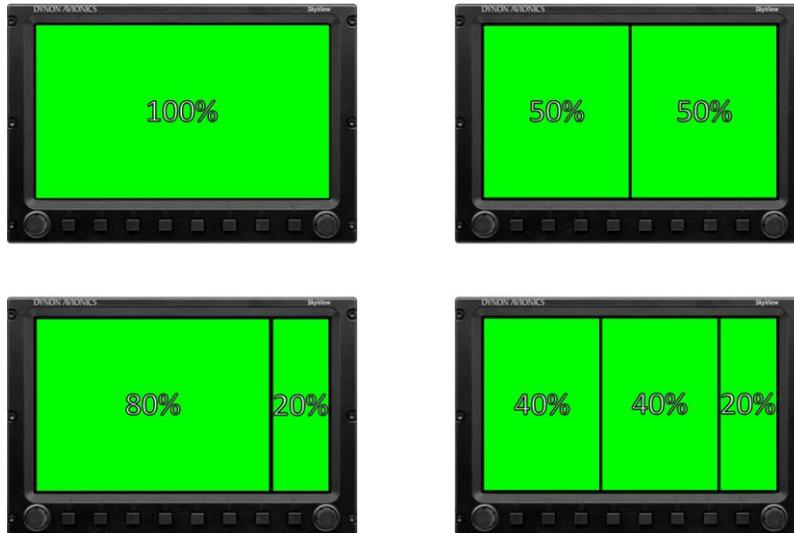
**Figure 6—Example Screen Layout Configurations**
