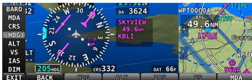
Figure 13–Autopilot Control Bugs Grayed Out
