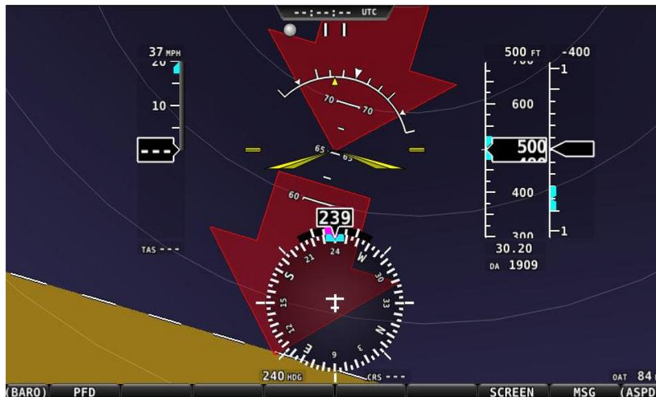
Figure 35–Extreme Pitch Warning Indicator Arrows
