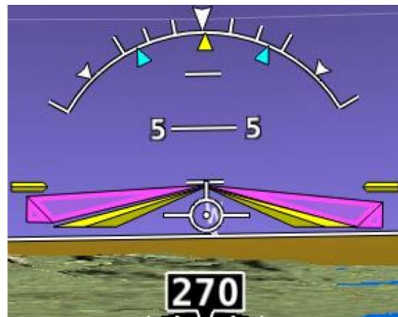
**Figure 165 - Single Cue / Inverted-V with Autopilot Servos Not Engaged**
