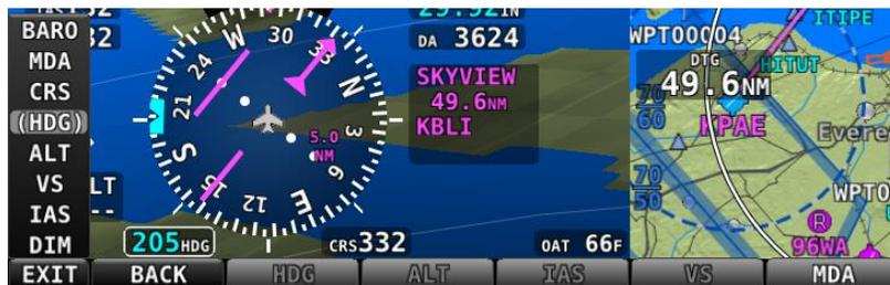
Figure 13–Autopilot Control Bugs Grayed Out
