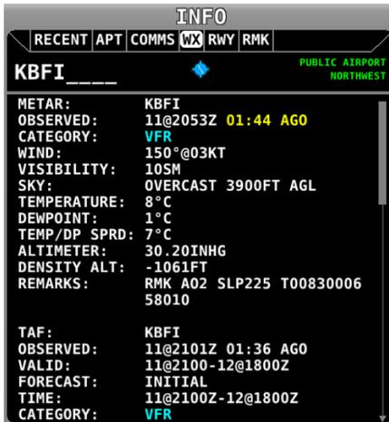
Figure 124 - METAR - Decoded
